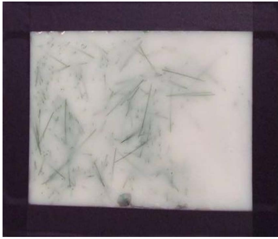
FIG. 1. (Color online) A phantom containing nylon filaments.
